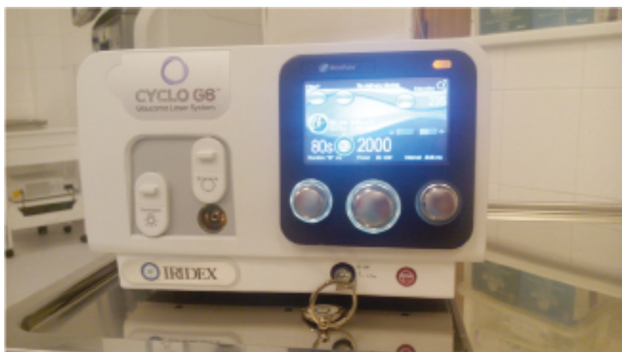
Fig. 1. Laser Cyclo G6 from Iridex company. Setting of the parameters can be seen on the monitor of the instrument: length of application 80 seconds, energy 2000 mW
