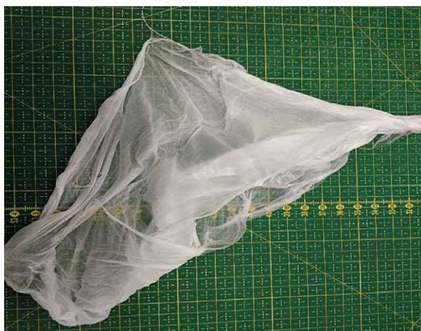
Figure 3. Macroscopic image of Povidone-iodine functionalized nanofibers
