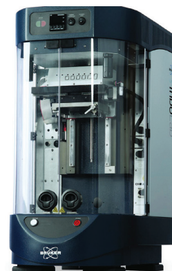
Fig. 1 Bruker UMT TriboLab universal tribometer (source: https://www.blue-scientific.com/brukey-umt-tribolab )
