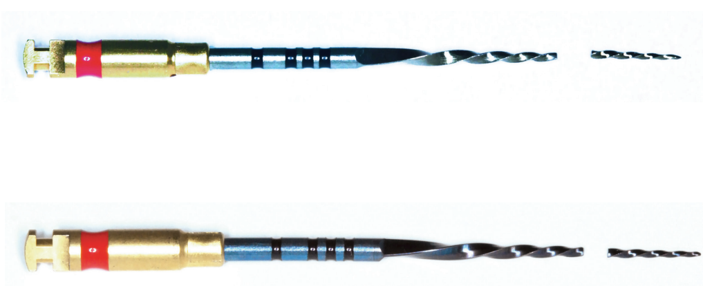
Fig. 3 Instrument Unicone – with separated fragment
