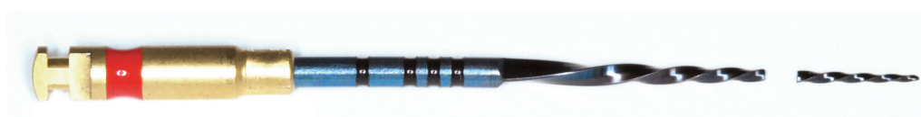
Fig. 4 Instrument Unicone Plus – with separated fragment
