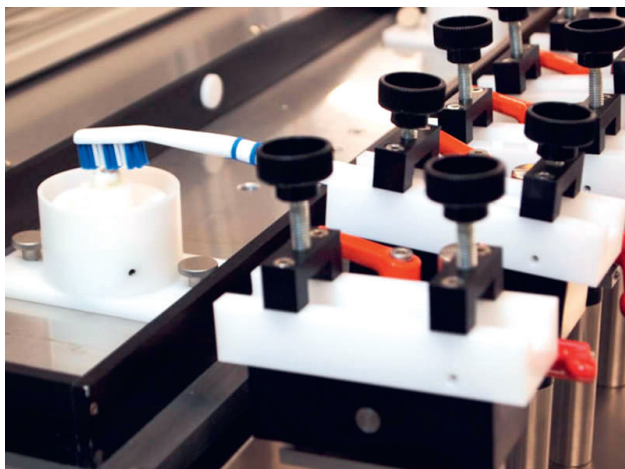
Obr. 3 Simulátor zubního kartáčku - toothbrushing machine [http://sdm-gmbh.de/en/products/toothbrush-simulation-zm-38-and-zm-312.html]
