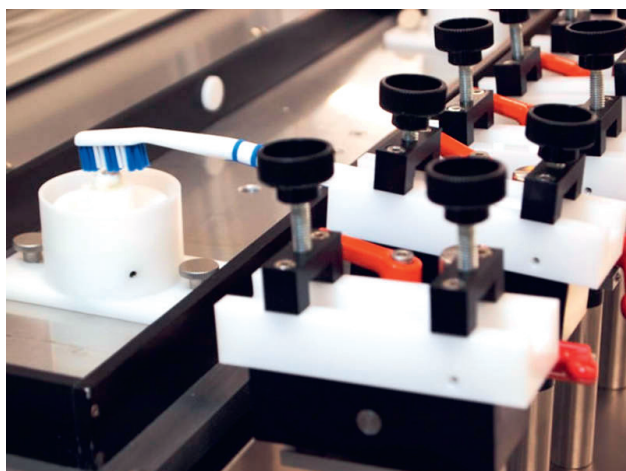
Obr. 3 Simulátor zubního kartáčku - toothbrushing machine [http://sdm-gmbh.de/en/products/toothbrush-simulation-zm-38-and-zm-312.html]
