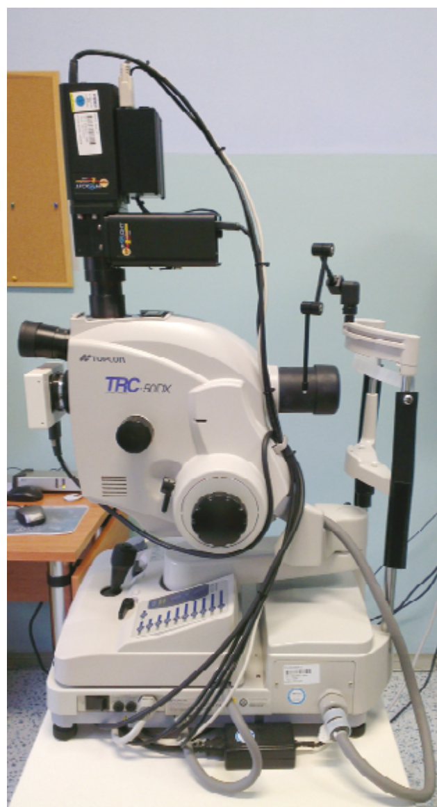
Fig. 1. Retinal oximeter Oxymap T1 (black instrument above) placed on Topcon retinal camera
