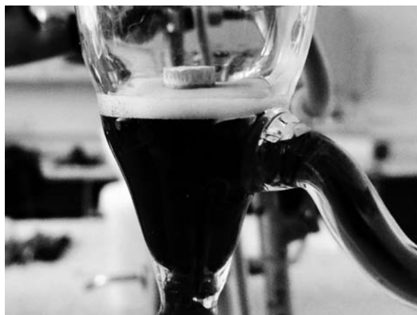
Fig. 1. Water absorption rate test of tablet
